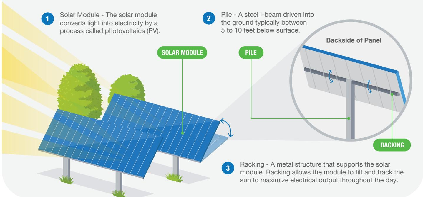
**3** Racking - A metal structure that supports the solar module. Racking allows the module to tilt and track the sun to maximize electrical output throughout the day.
