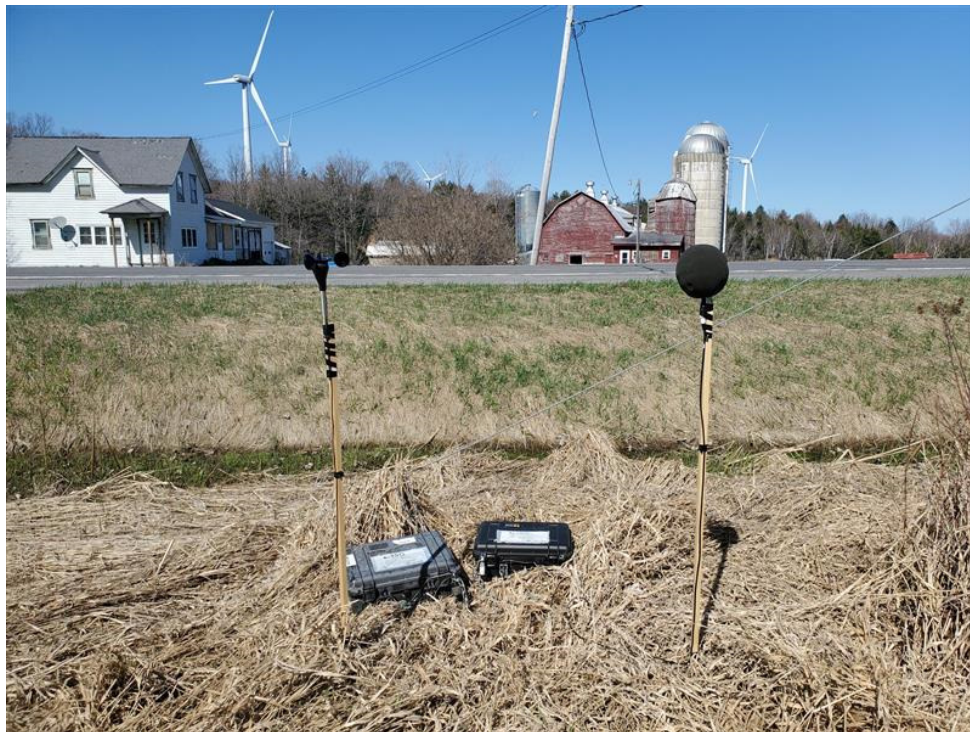
Figure 1: Example Setup of Noise Monitoring Equipment
