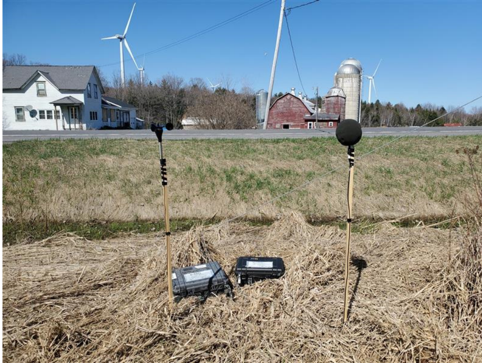
Figure 1: Example Setup of Noise Monitoring Equipment
